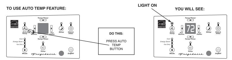
**Note:** Fan speed starts at High Speed and adjusts to a slower speed as the room temperature dictates. For example if the room doesn't get too warm, it will stay at the slowest speed. If the room temperature rises quickly, such as a door being opened, it will automatically go to the highest speed. The fan speeds will re-adjust back to the slowest speed as the room returns to the original set temperature.
